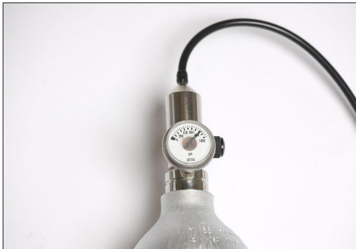
Figure 26 Flow Regulator Fitted to Calibration Bottle
