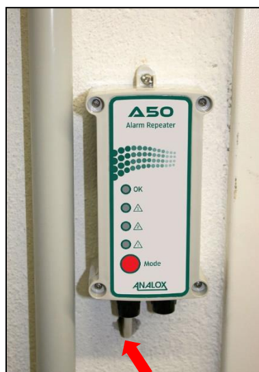
Repeater connections (Hard wired shown)
