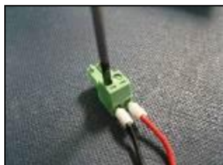
4) Secure using a terminal driver
